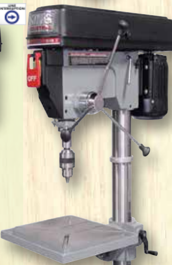
Safety guard with limit switch protection
