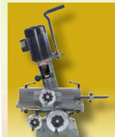
Head tilts from 0° to 30° to the right and left for angle mortise cuts
